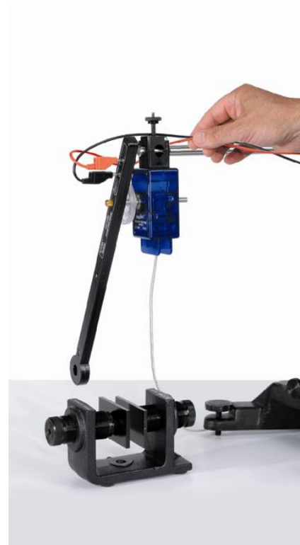
Figure 4: Coil Passes through Magnet
