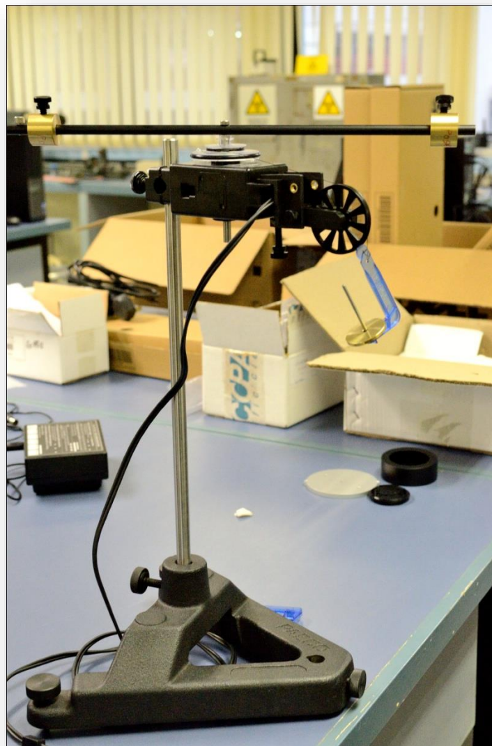
Fig. 2: Physical set-up of the Rotary Motion Sensor and the Pulley for Experiment 1
