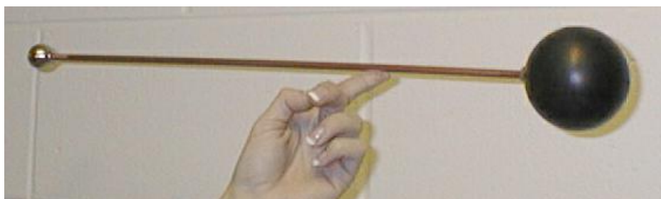
Figure 3. Experimental method to find the position of center of mass
