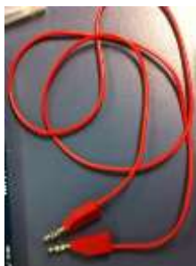
Figure 12: A wire for shorting the capacitor
