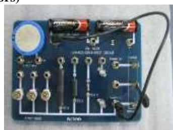
Figure 7: Connecting the wire from negative terminal of 3V battery to the switch
