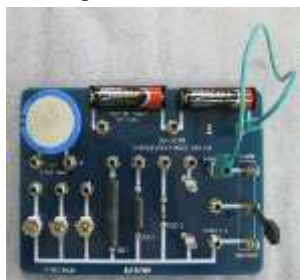
Figure 5: Connecting the wire from positive terminal of 3V battery to the switch
