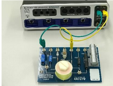
Figure 24. Connecting power source of the Interface to the Circuit board as LRC series circuit
