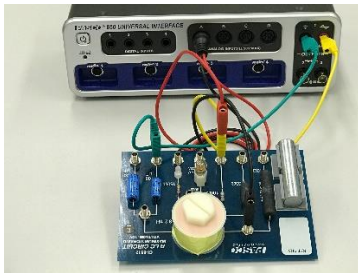
Figure 25. Voltage Sensor in Channel A for measuring p.d. across resistor, V_R
