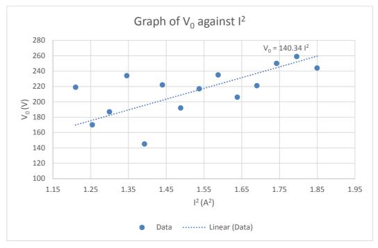
From the graph, the slope is 140.34. Since the slope is equal to  $\frac{e}{m} \left(\frac{N\mu_0 r}{R}\right)^2 \frac{1}{2(5/4)^3}$ , the charge to mass ratio is obtained:
