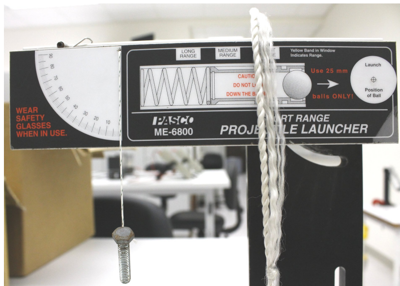
Figure 1: This is a projectile launcher that can be set at any angle ranging between 0^\circ to 90^\circ . A plumb bob made up of a hex bolt and a string can assist you in reading off the projectile angle \theta .
