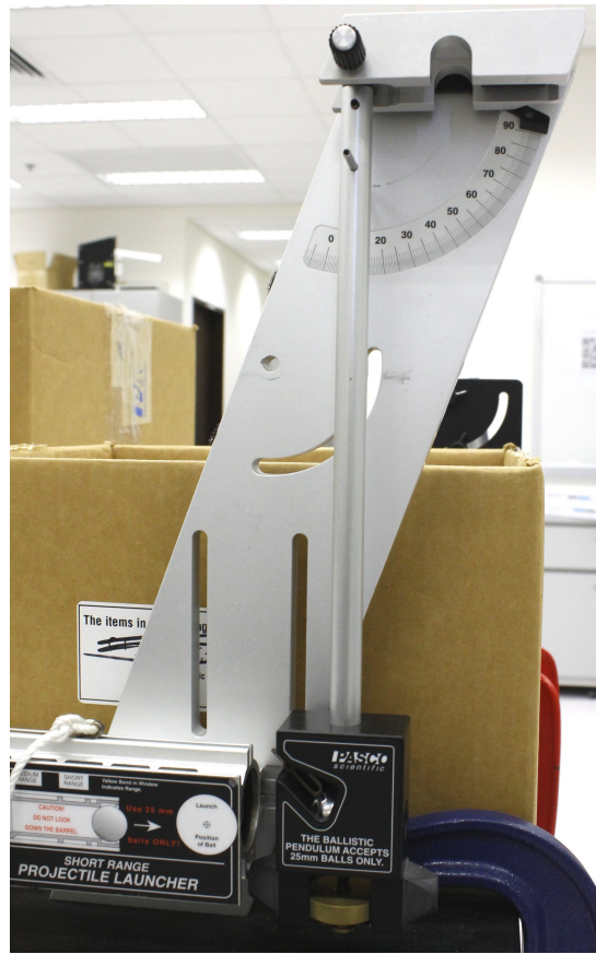
Figure 2: After being launched, the metal ball will be trapped within the ballistic pendulum. This pendulum-ball system will then swing upward to some angle.
