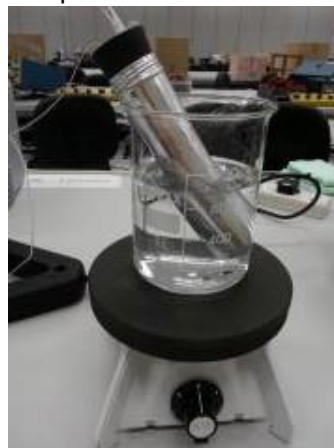
Figure 4c – Air chamber with temperature sensor and pressure sensor on the hot plate
