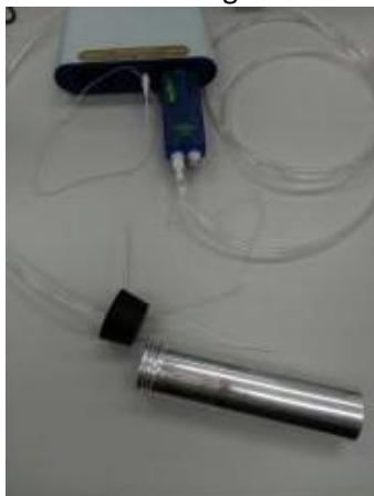
Figure 4b – Temperature sensor and pressure sensor fitting with the two-holed stopper
