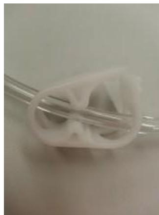
Figure 3 – Shut-off valve on tubing
