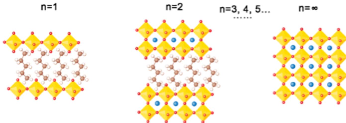
Figure 1. Illustration of multidimensionality in  $A_2A'_{n-1}B_nX_{3n+1}$  perovskite materials
