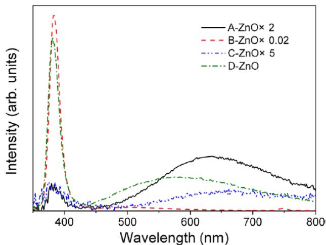
Figure 2. Photoluminescence spectra of different ZnO nanoparticles.
