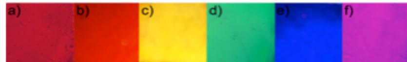
Photos of different BA-MA and BA-Cs lead and tin perovskite thin films under UV illumination
