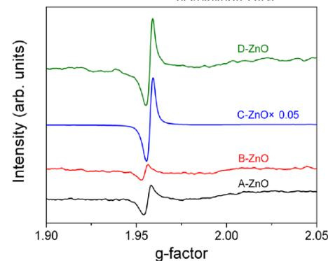
Figure 5. Electron spin resonance spectra for different ZnO nanoparticles.
