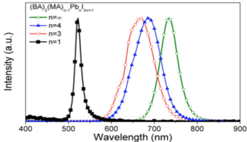
PL spectra of  $(\text{BA})_2(\text{MA})_{n-1}\text{Pb}_n\text{Br}_{3n+1}$  with various  $n$  values
