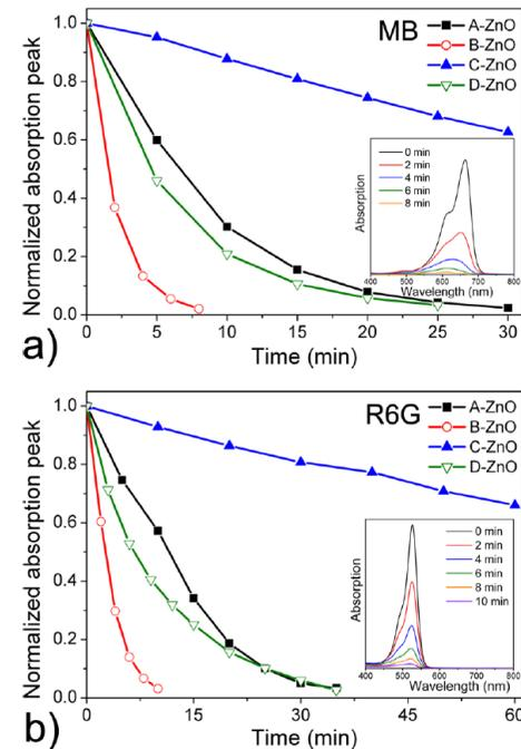
Figure 8. Degradation curves of cationic dyes for different ZnO nanoparticles (a) methylene blue and (b) rhodamine 6G. The insets show absorption spectra at different times corresponding to the fastest degradation curve
