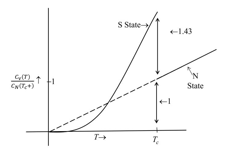
Specific heat normalized to N-state value at  $T_{\!c}$
