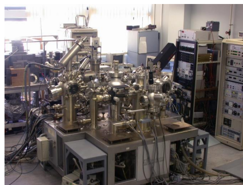
A multi-chamber ultrahigh vacuum system consisted of multi-facilities such as MBE, UPS, LEED and STM
