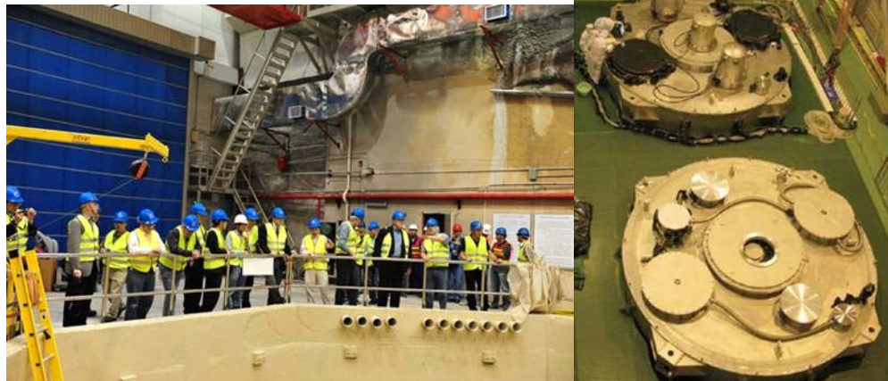
大亞灣中微子振蕩實驗 - 大亞灣近端地下實驗室（左圖）已建造完成，而首兩個反中微子探測器（右圖）亦已完成裝嵌，並通過一系列測試。The Daya Bay Neutrino Oscillation Experiment - the Daya Bay Near Site underground experimental hall (left) is ready for use, and the first pair of anti-neutrino detectors (right) have been assembled and tested.
